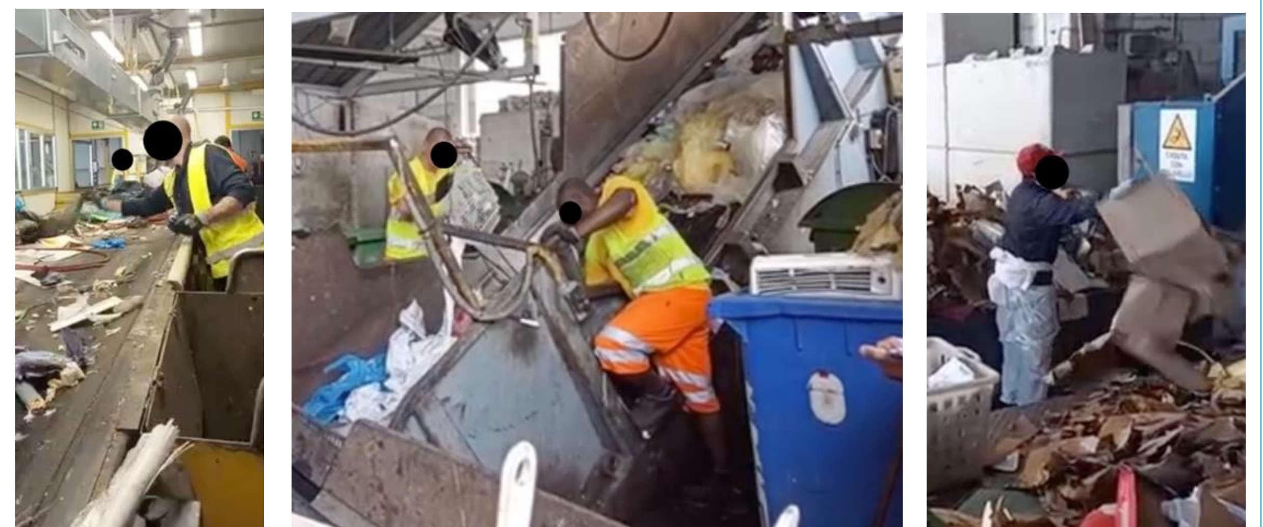
Fig. 3: Workers engaged in manual sorting by conveyor belt placed horizontally (left), by conveyor belt placed obliquely (centre) and on the ground (right).
